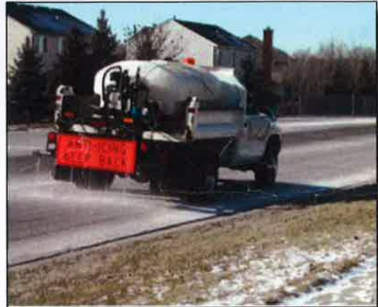
Typical anti-icing equipment for roadways.
