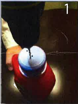
1 Drill eight to ten 1/8" holes into the top of the cap on whatever container you choose.
